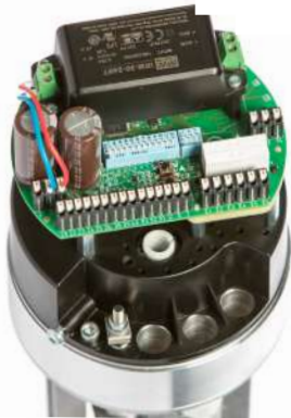
View without cover showing the baelz 7022 circuit board (230 V version)
